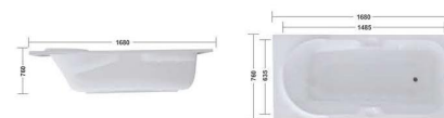
Length 1680mm | Breadths 760mm Depth 390mm | Waste Hole Distance from wall 340mm WBT-004
